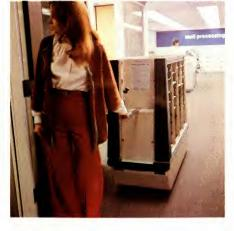
Mailmobile can be easily maneuvered by means of a steering handle with integral hand-operated grip switch. This switch controls both forward and reverse movement of the unit. Handle retracts into unit for automatic operation.
